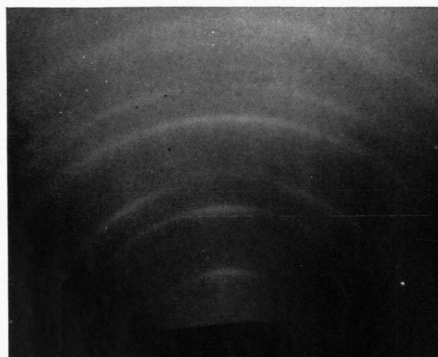
Fig. 3. Same as Fig. 2, but now \sqrt{3} and \sqrt{8} rings are equally strong at the centre, \sqrt{12} and \sqrt{27} rings have just begun to appear at the centre and \sqrt{18} ring is almost uniformly intense. This shows a weakening of 110 orientation and an increase of 111 orientation as compared with Fig. 2.
